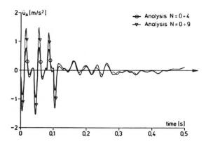
Figure 4. Horizontal acceleration of the shell model at reference point A.
