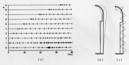
Figure 2. Eigenfrequencies of the shell model (a); mode shape N=1, mode 2, 2.6 Hz (b); mode shape N=2, mode 15, 79 Hz (c).
